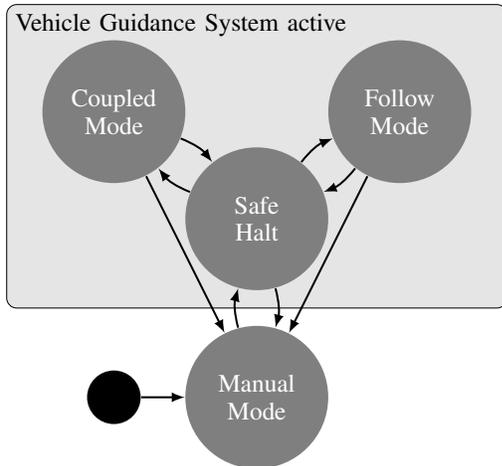
Fig. 2. Modes of Operation of the Planned System
